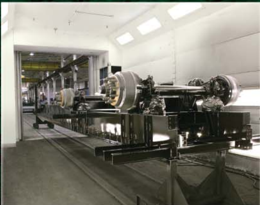
Electrostatically applied plural component urethane top coat provides superior resistance to corrosion.
